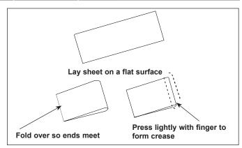
Figure 3. Folding Release Sheet
